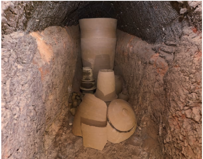
Jar-coffin fragments are put in front of a jar-coffin to block the flames.
