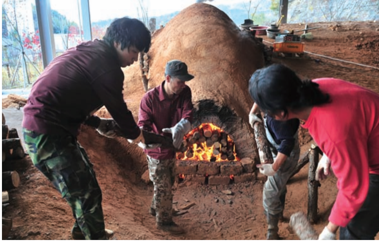
Filling the entrance of the kiln with firewood to make a large fire, which is the last step of kiln firing
