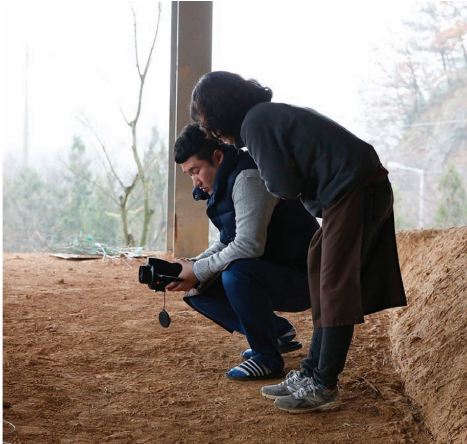
Taking images using an infrared thermal imaging camera A thermal imaging camera is used to identify heat flow inside the kiln.
