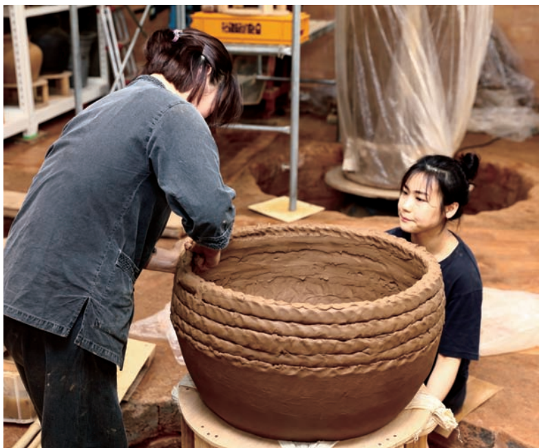
Make a groove on the connecting part of the lower body and stack clay strings to make a body.
