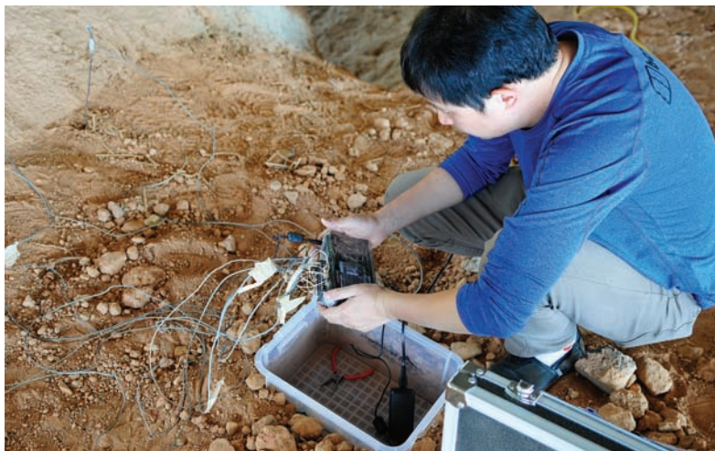
Installing multi-channel thermometers
