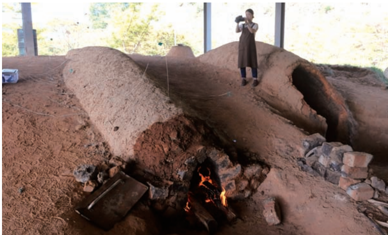
Researcher Lee, Hye-yeon recording the change in kiln temperature using an infrared thermal imaging camera
