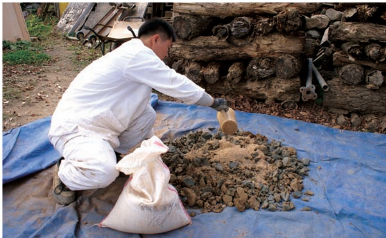
Mix clay and temper and blend them by adding water.
