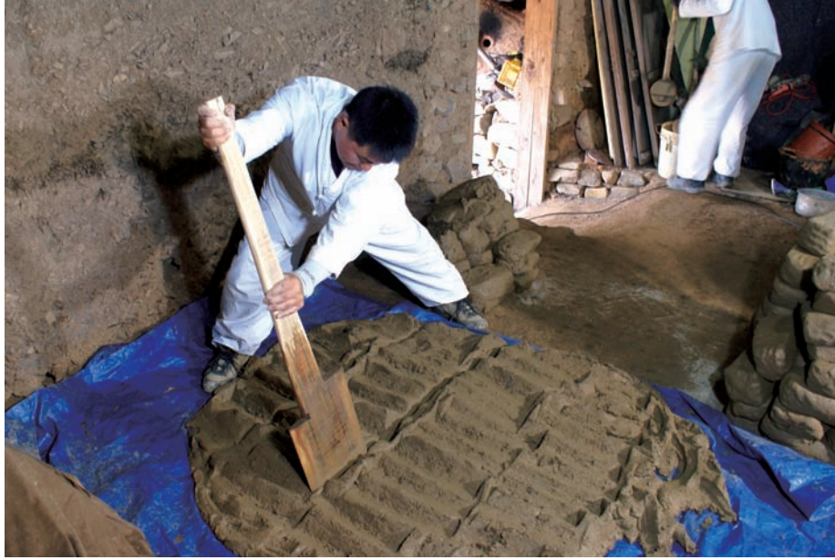
Assistant Researcher Sung, Yun-gil mixing and kneading clay using a wood shovel
