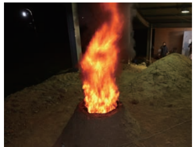
When the kiln reaches the highest temperature, flames burst out of the chimney.
