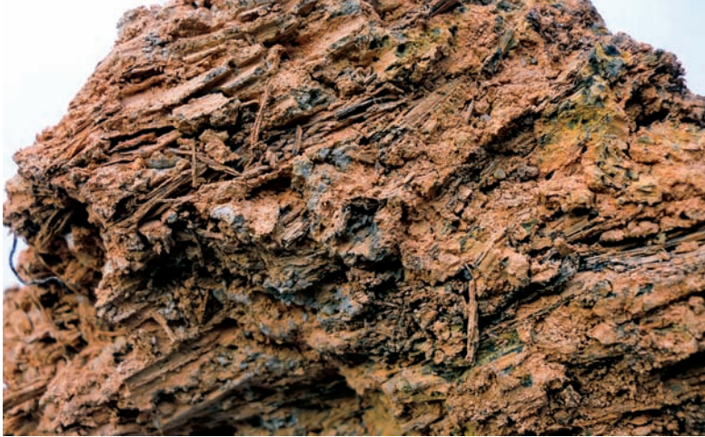
Traces of grass found in a ceiling piece of a kiln site in Oryang-dong, Naju
